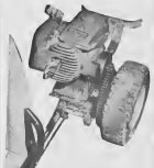
THIS IS the heart of a kart. A two-stroke engine, this tiny "mill" puts out all of two-and-one-half horsepower.
